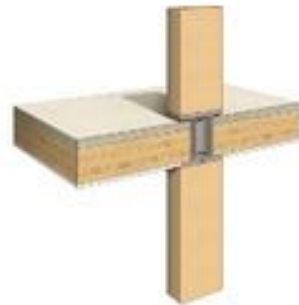
partial encapsulation during construction
