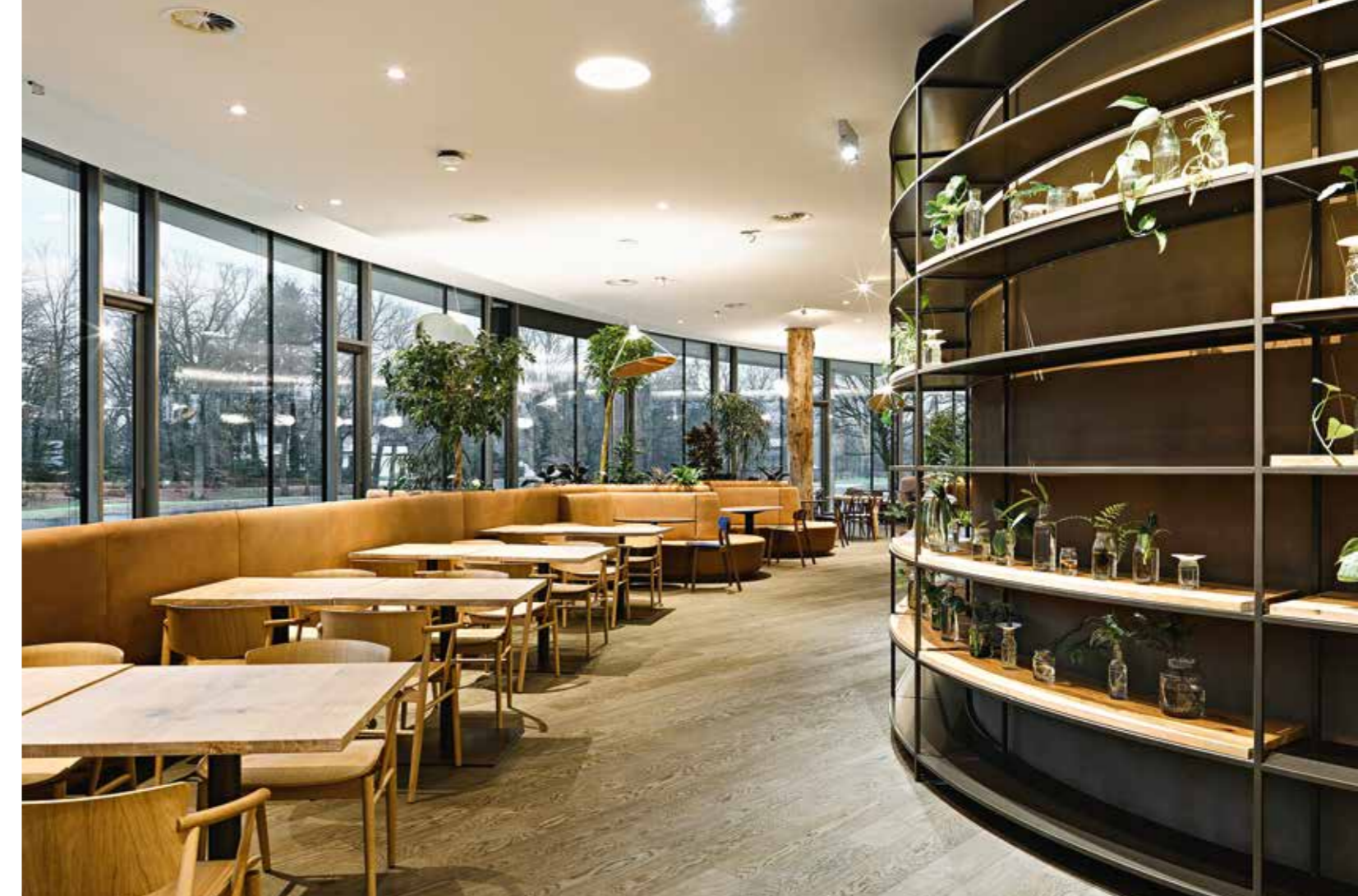
The building already contains recycled material, including roof beams and the floor in the restaurant. Tree trunks appear throughout the building, serving both a visual and a load-bearing function.
