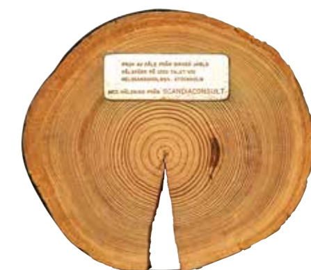
Cross-section of a sample post taken from Birger Jarl's wooden sea defences, dating from the 1250s. The healthy, intact wood has split as it has dried out, but only after more than 700 years in the ground.
