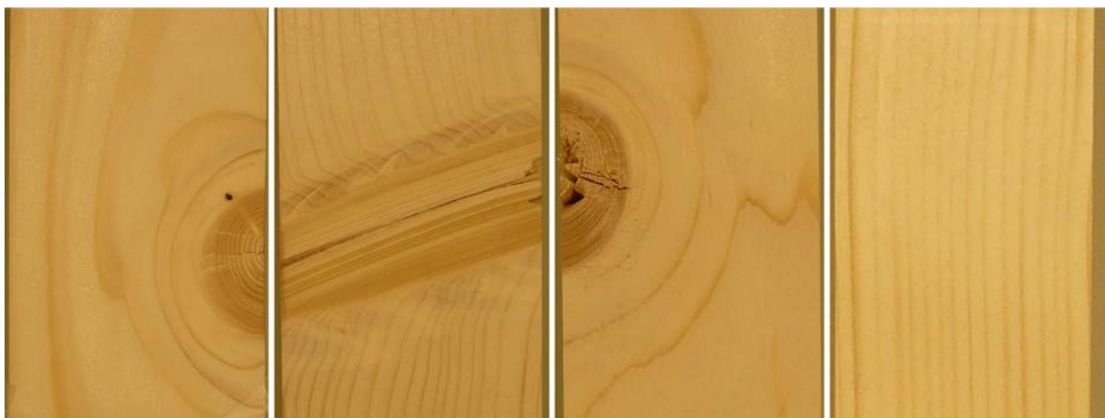
Figure 2.8: A knot seen from all four sides of a wood specimen 45 x 45 mm in square section (Photo Bertil Enquist).
