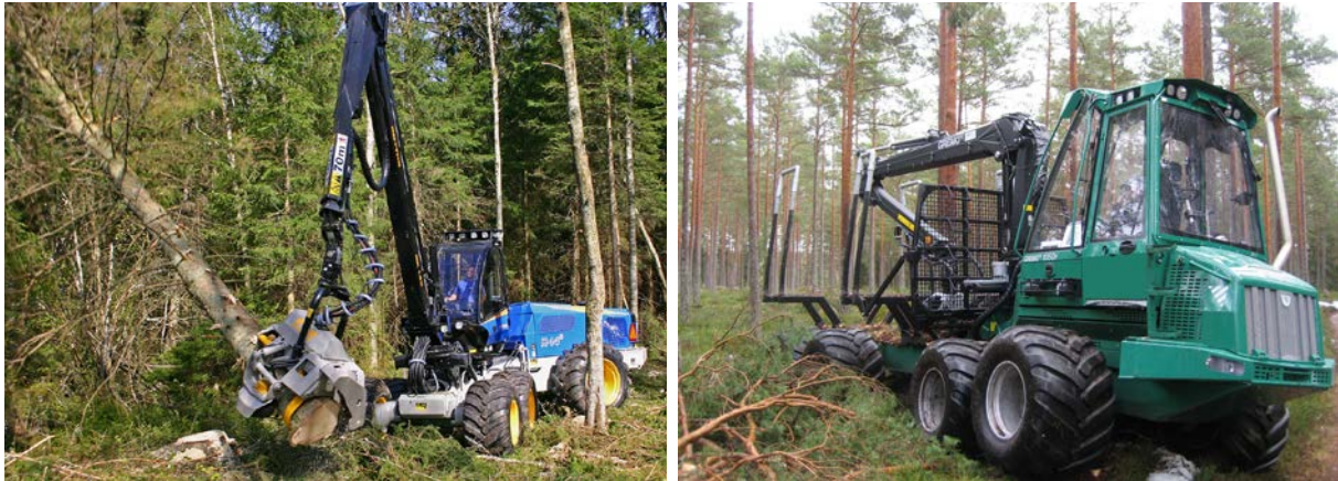
Figure 2.3: Harvester and logger in action in the forest (Photo courtesy of left: Rottne industri AB and right: Gremo AB).
