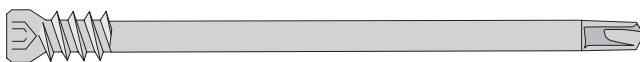
Figure 4.19: Special fastener designed for steel-to-timber joints enabling drilling the hole and mounting the fastener in one working moment.
